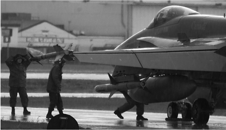
3.6. Canadian armorers working in pouring rain carry an AIM9M8/9 Sidewinder Missile that locks onto and tracks Infrared energy emitted by an enemy aircraft. Photo courtesy of the Department of National Defence.
