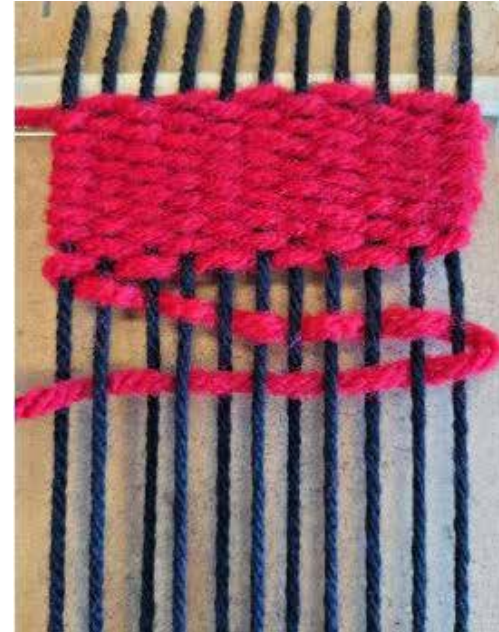
On this home-made loom, the black threads are the warp, and the red threads are the weft.
